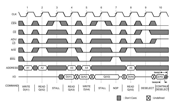
**Note**: 1. The IGNORE CLOCK EDGE or STALL cycle (clock 3) illustrates  $\overline{\text{CEN}}$  being used to create a "pause." A WRITE is not performed during this cycle.
